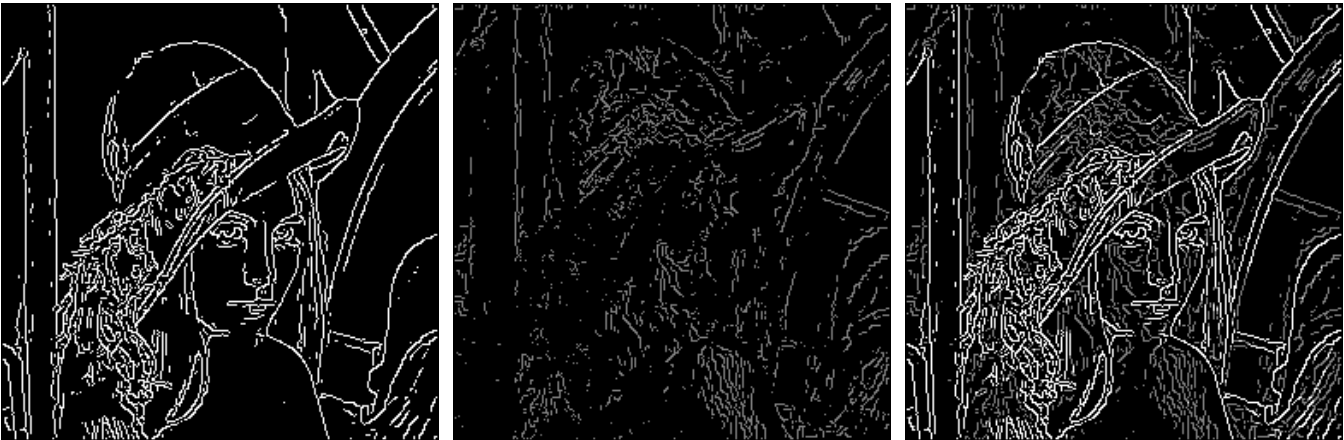
Figure P.8: Step 4: Double threshold. The strong pixels (left), the weak pixels (middle), and the combined (right).
