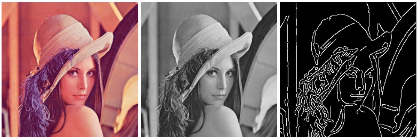
Figure P.1: Edge detection, using the built-in function “edge”, which is not perfect but somewhat acceptable .
