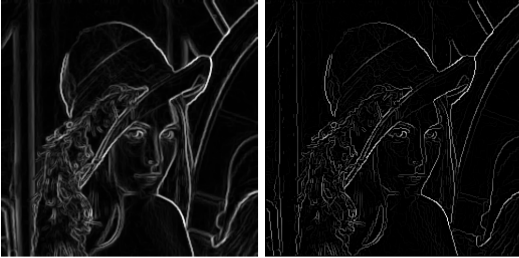
Figure P.7: Step 3: Non-maximum suppression. The Sobel gradient in Figure P.5 (left) and the non-maximum suppressed (right).
